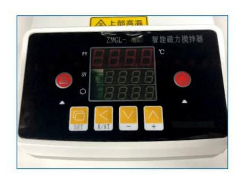
Fuzzy PID temperature control, dual-screen digital display, high precision, little over temperature, and break protection function.
